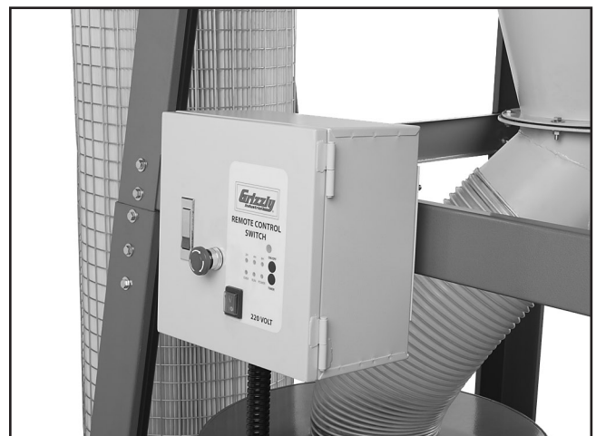
Figure 41. Model G0638 control box mounted.
